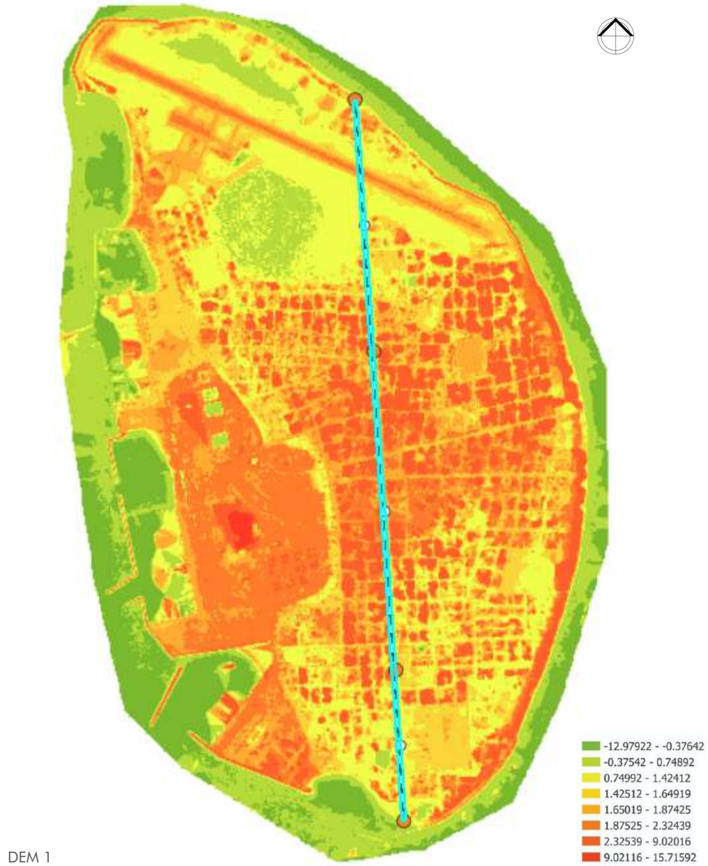
Figure 22. The DEM1 , shows the color scale where the highest surfaces are red in color and the lower surfaces are green in color. The reclaimed land, eastern ridge and the airport are higher in elevation than the rest of the island and the burrow areas for the reclamation, the mangroves and the roads are lower in elevation than the rest of the island.
